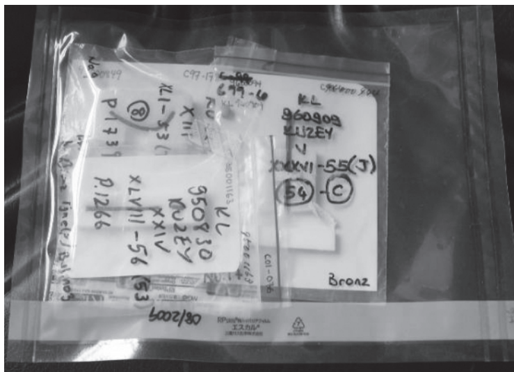
Fig.3 and Fig.4 Completed RP System™ storage bags, each containing metal artifacts, RP Agent and an oxygen indicator. The objects and oxygen indicator are placed within the bag such that they are easily visible and the date of enclosure is inscribed on the writing strip.
