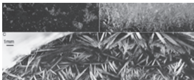
Fig.3.3a Crystal formation of cyclododecane in different solvents
