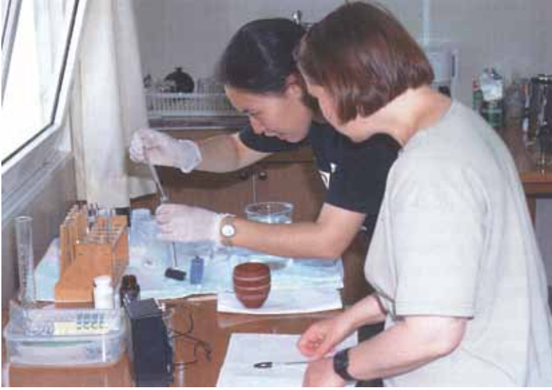
Figure 3: Measuring the conductivity of bath water during the desalination of excavated ceramics. Kaman-Kalehöyük, Turkey.
